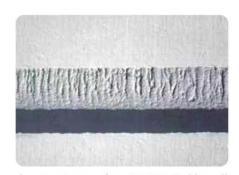
Laser cut no surface treatment side wall
