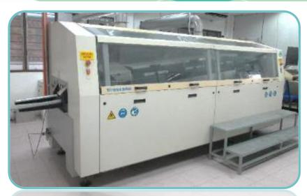
**Vitronics Soltec Wave Soldering Machine**
