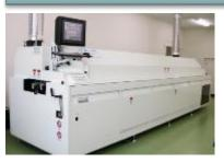
**Reflow Soldering Machine**
