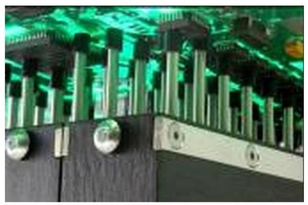
Example of adaptable PCB support in use
