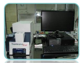
RIGAKU Differential Scanning Calorimeter
