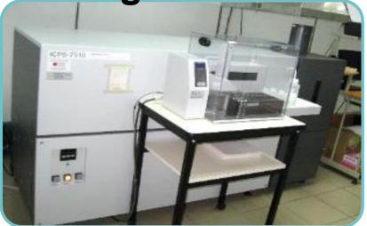
**SHIMADZU ICPS Emission Spectrometer**
